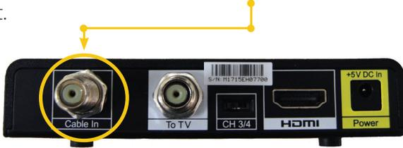
2. Next, take the white coax cable that came in your installation box and screw one end into the back of the TV, where you just removed the old cable. Place the other end into the back of the DTA box in the spot labeled "To TV."
